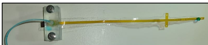
Figure 1. Bioelectronic implant bonded to a microfluidic channel, enabling combined electrical stimulation and localized drug delivery in rats.
