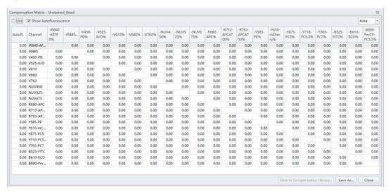
**2** In the Keywords column, the corresponding compensation values can be selected for each channel. The compensation values of the same keyword can also be selected using the drop-down menus in the Keywords column.
