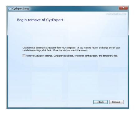
**IMPORTANT** If the *Remove CytExpert settings, CytExpert database, cytometer configuration, and temporary files* checkbox is checked, your settings, database, configuration files, and temporary files will be overwritten and you will need to reinstall your cytometer configuration and restore any databases you might have.
